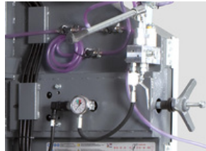
Hydraulic saw blade tensioner 1000H40
