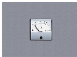
Ammeter - blade load indicator
